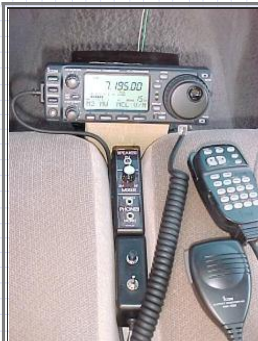
Remote Control The lower box is the remote control that plugs into the ATAS
